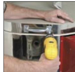
C. Remove the Lid Brace, Lid Brace Pad, and Lid Brace Guide
